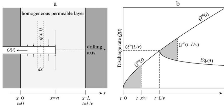
**Figure 1. Tunnel drilled through a subvertical permeable layer. (a) Nonuniform specific discharge resulting from progressive drilling. (b) Transient discharge  $Q(t)$  as expressed in Equation 3 with maximum at  $t = L/v$ .**
