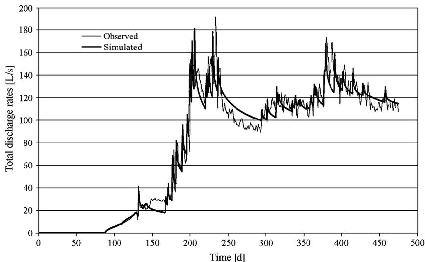
**Figure 4. Discharge rates into the Modane exploratory tunnel. Comparison of observed values with the analytical simulation using the detailed drilling history (model 2, 180 sectors).**
