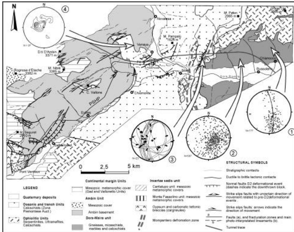
Figure 1: Geological sketch map of the studied area. Also includes the lower hemisphere stereograms of some significant structural features and the dead reckoning plot of the Pont Ventoux – Susa Hydropower Plant.
