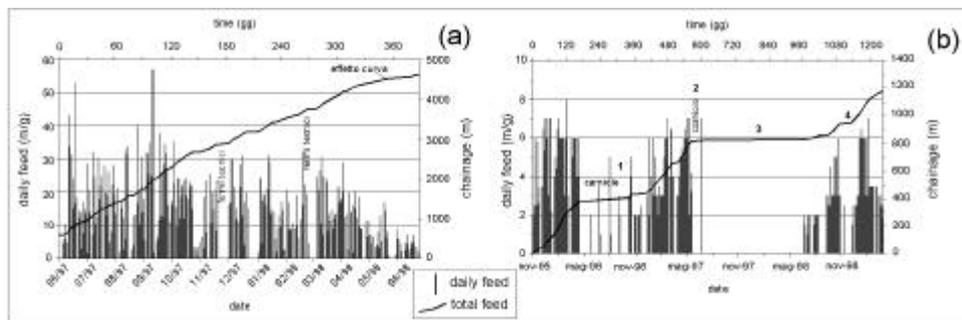
Figure. 4: Diagrams showing the excavation performances during the construction of the Pont Ventoux – Susa Hydropower Plant; graph (a) shows D&B performances in the structural domain 4 and the plateau n. 1 and 3 correspond to the intersection with the most important shear zones; graph (b) show open TBM performances in typical conditions of structural domain 5. Histograms represents the daily performances.
