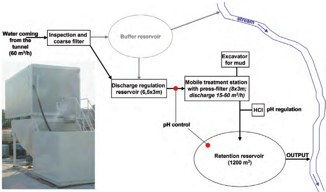
Fig. 5: Water treatment plant installed on the work site to separate suspended mineral particles after flocculation and sedimentation.
